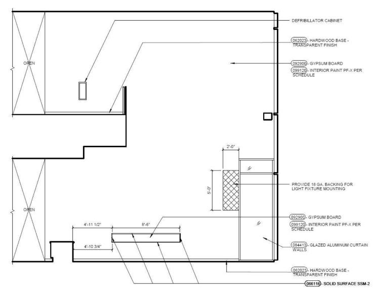
Figure 13: Rock Wall Area West Elevation
