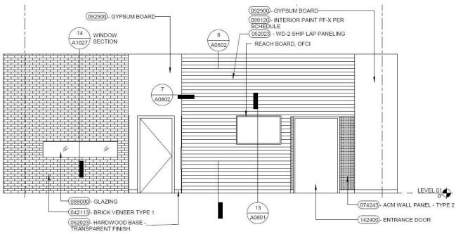
Figure 6: Control Counter North Elevation
