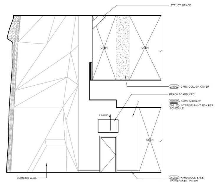
Figure 15: Rock Wall East Elevation
